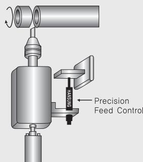
CSC as drilling and cutting fixture
