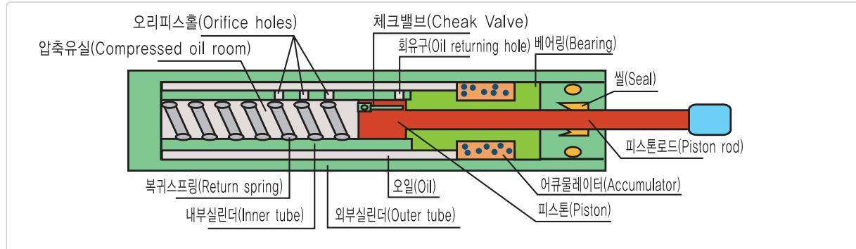
Internal construction of Shock Absorber
