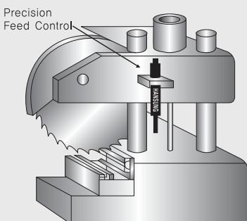
CSC as sawing and milling fixture
