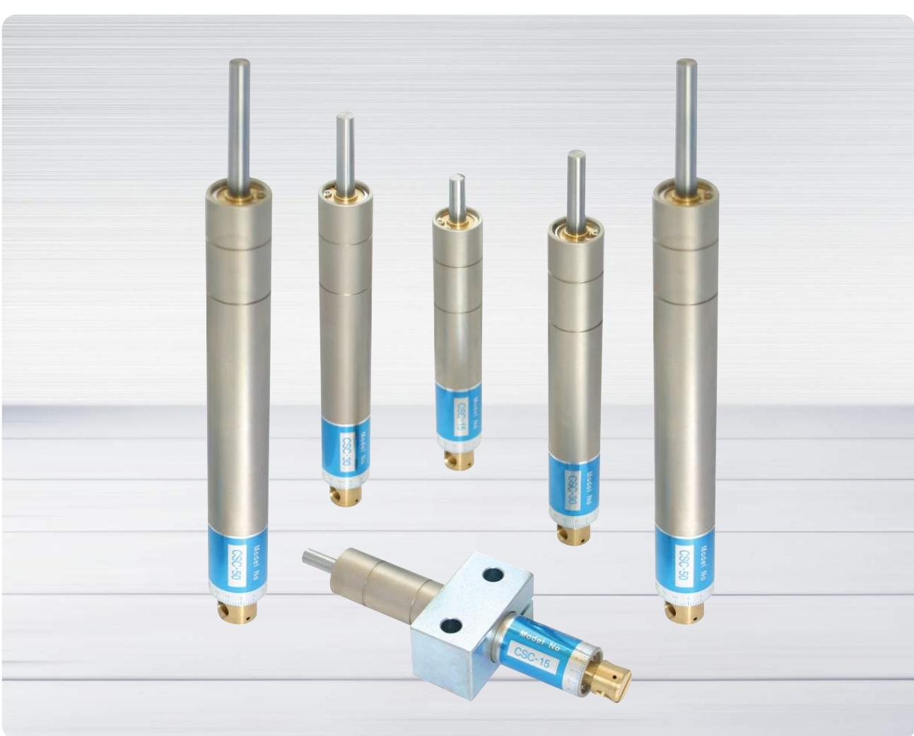
HANSUNG have 3 kinds of CSC model which control the speed of both light and heavy loads with smooth and consistent capacities. They are available in stroke lengths of 15mm, 30mm, 50mm with capacities from 2.5Kg to 150Kg force.
